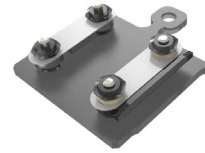
Direct current sample plate e.g. for Si sample preparation.
