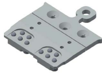
Sample plate with multiple electrical contacts.
